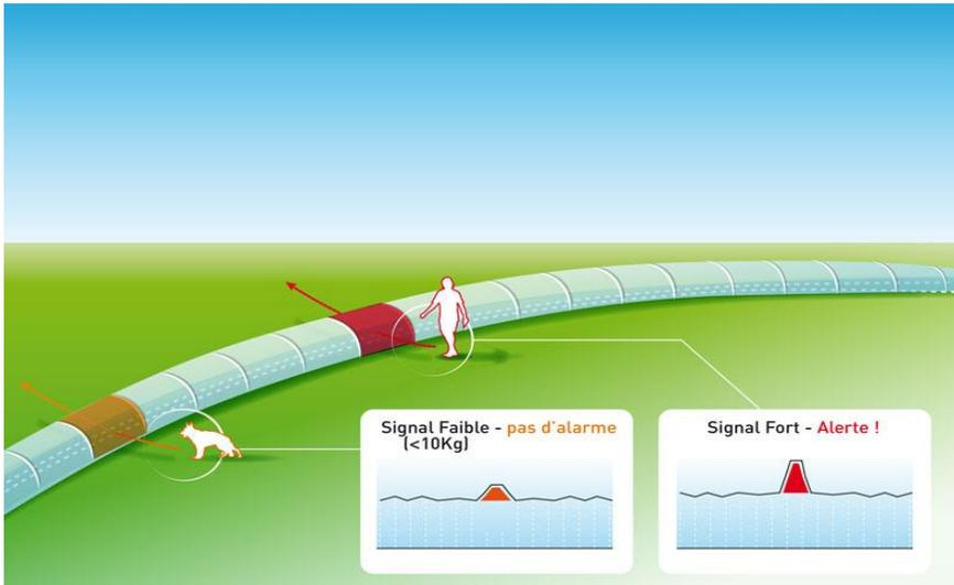
Detector cables are intelligent buried detection systems. They are composed of two microwave coaxial cables buried underground in the same trench and therefore invisible.
